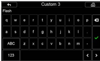
Using the touch keyboard to rename the Custom Setup
