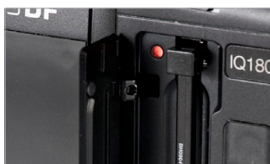
Installing and removing the CF card
